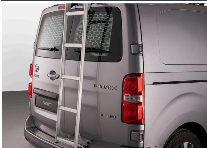
The fixed ladder is ideal for easy and safe access to your Toyota aluminium or steel roof rack.
