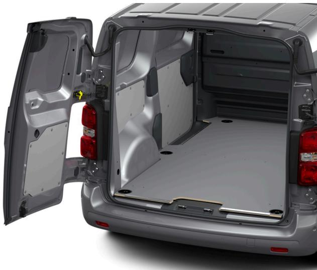
Available in Plywood or a 9mm or 12mm Textured Wood or a Pre-drilled 12mm Textured Wood for adding Premium Racking
