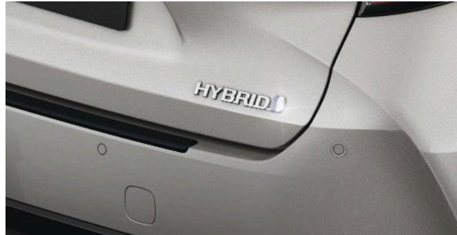
Rear parking sensor system with 4 ultrasonic sensors and an acoustic warning.
