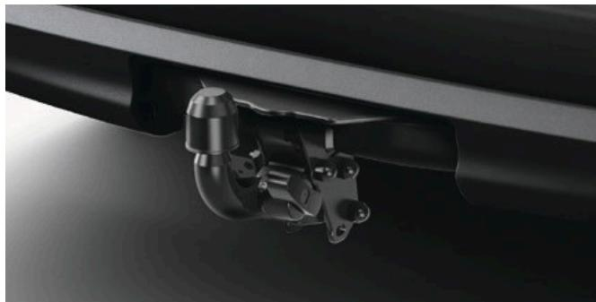
The towing hitch gives you ideal capacity to tow a trailer. It is designed for the Toyota Corolla Hatchback and has a tough anti-corrosion surface treatment.
